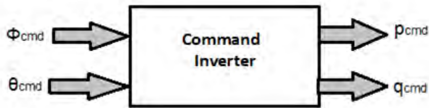
Figure 3: Command inverter block
