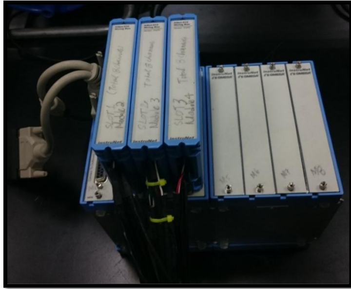
Figure 33: Data acquisition used with load cells and LVDT's
