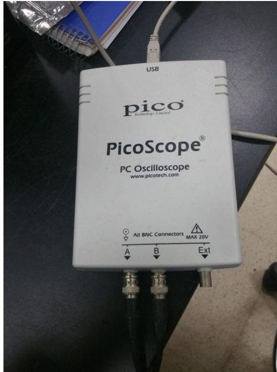
Figure 19: Pico Scope used for recording accelerometers output signals
