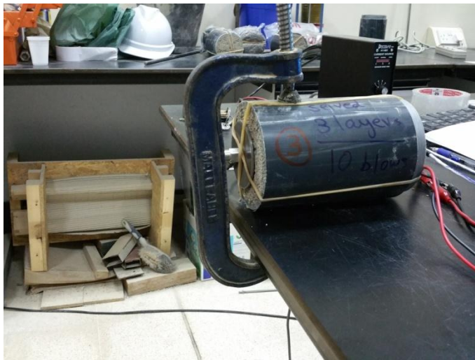
Figure 23: Clamping the soil specimen to a rigid table
