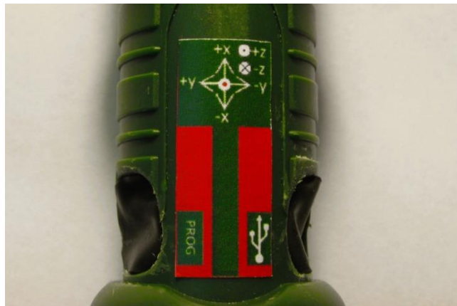
Figure 36: ZTID stickers showing accelerometer axes
