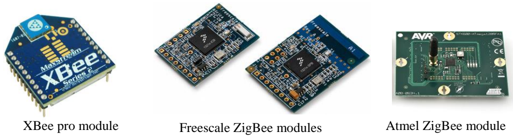
Figure 4: ZigBee network module options [19], [20], [21], and [22]
