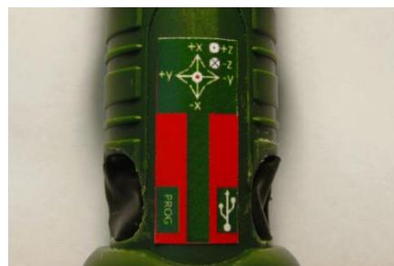
Figure 23: ZTID stickers showing accelerometer axes
