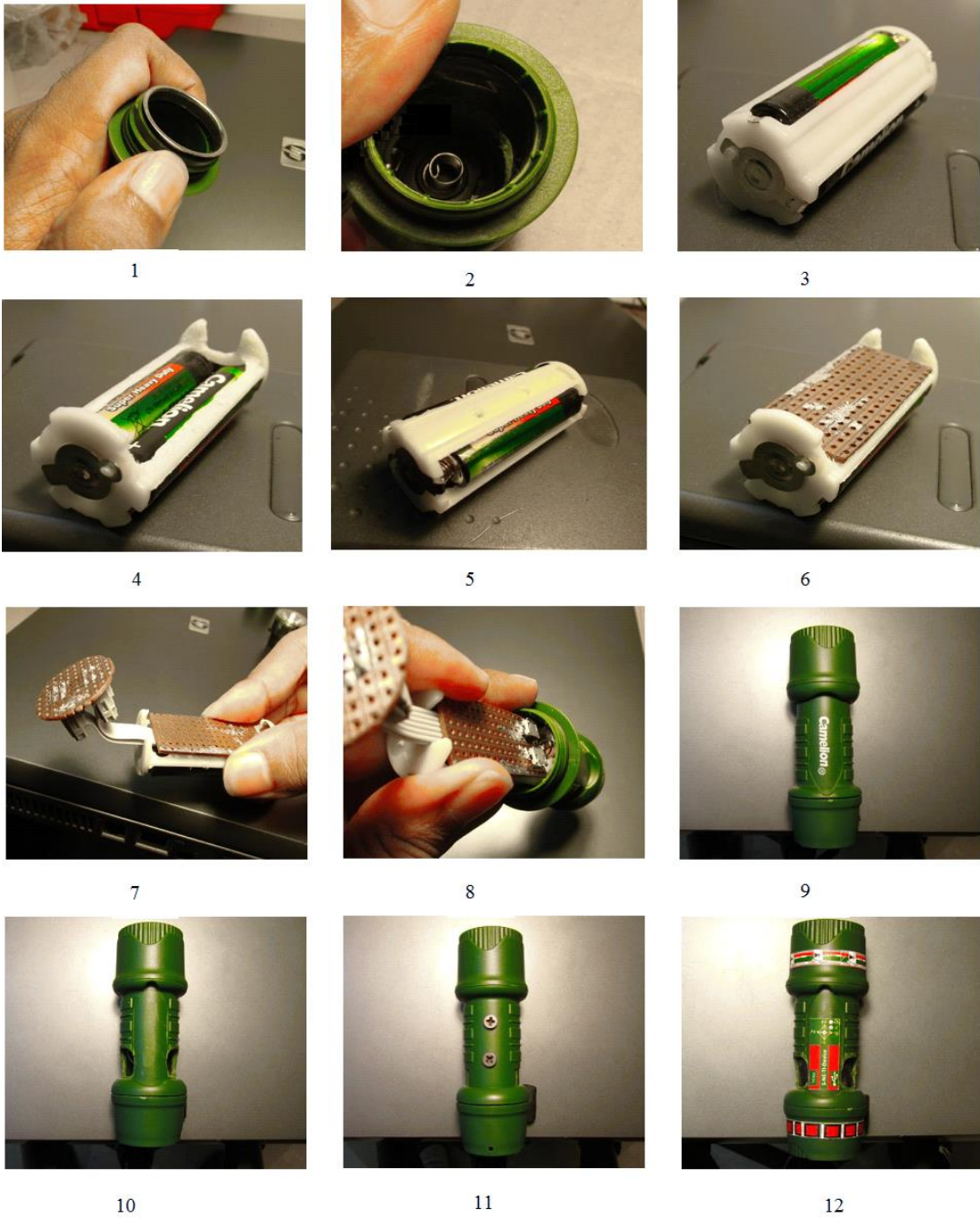
Figure 41: Casing modifications for RF-control-board
