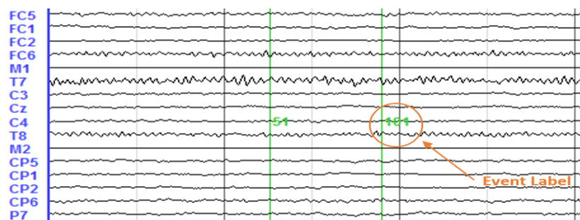
Figure 24: Event labels in EEG signal
