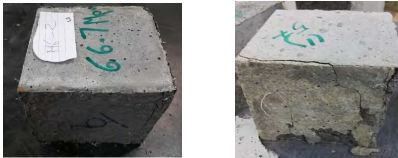
Figure 4.1: Typical failure mode of (a) Fiber reinforced concrete cubes, (b) Control sample.
