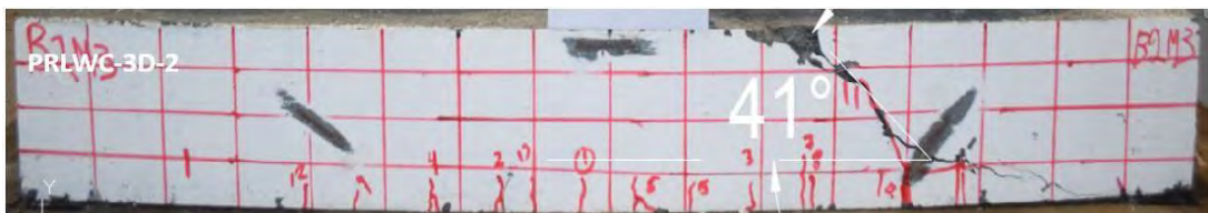
Figure 4.8: Mode of failure and shear angle of beam PRLWC-3D-2.
