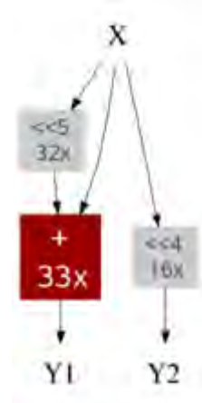
Figure 24: Block 9 in 1-D Gaussian Filter Block
