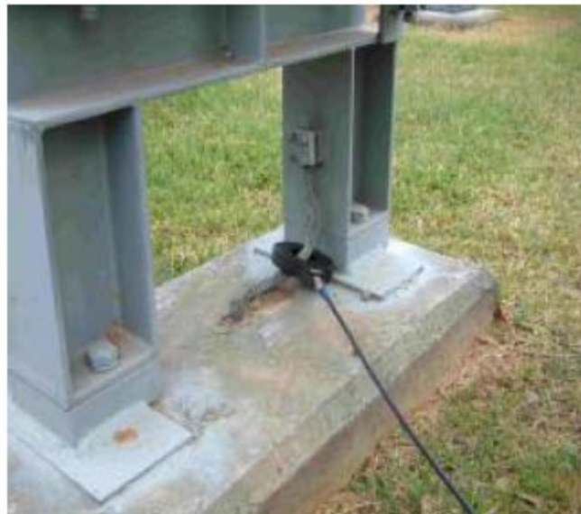
Figure 3: PD detection using HF-CT [6]
