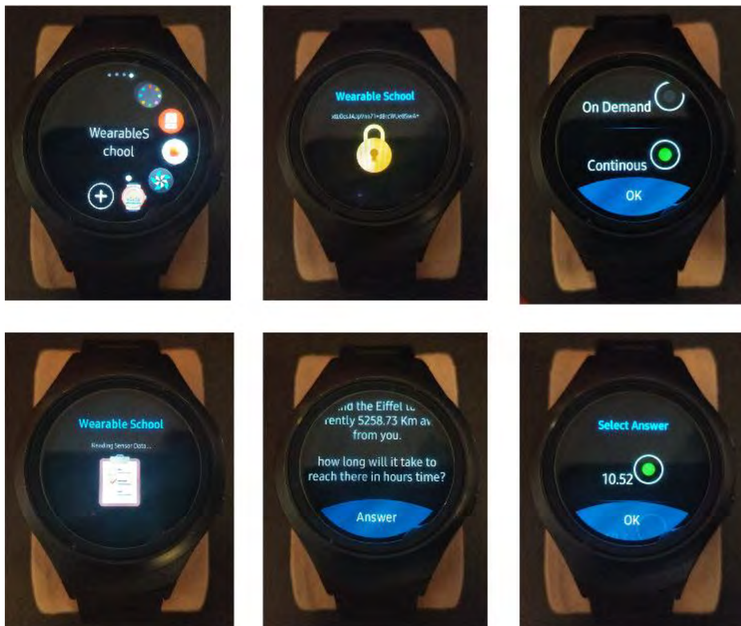
Figure 3.5: Sample in-situ question shown on smartwatch. Screenshots from left to right, and top to bottom show the user interface cycle throughout the application.
