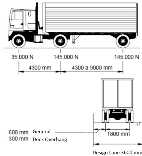
Figure 9: Characteristics of AASHTO LRFD design truck [4]
