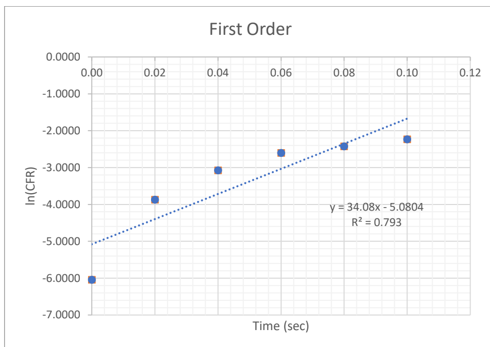
Figure 4.6: The fit of experimental data to the first-order model for non-folated micelles DOX release at 3.54 \text{ W/cm}^2 power density
