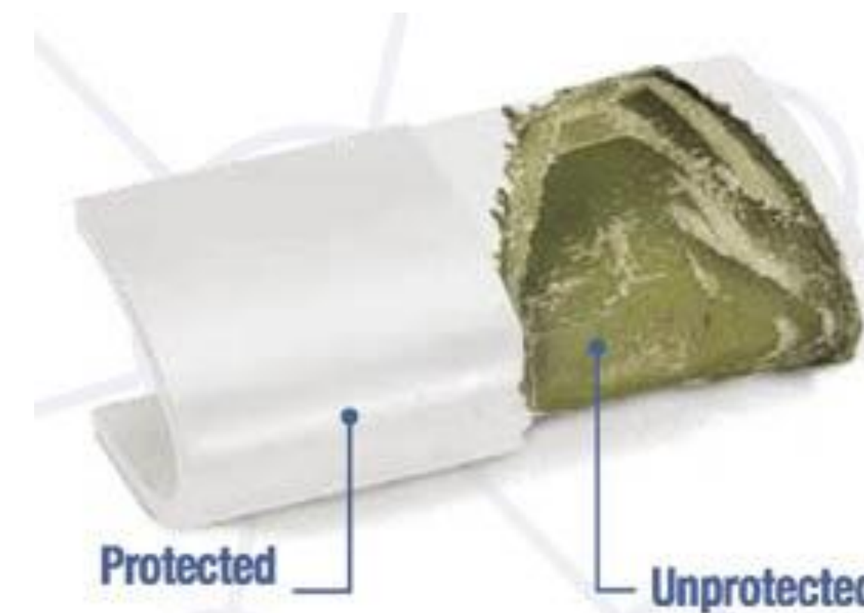
Figure2: Results of protection & non-protection on an airfoil [1]
