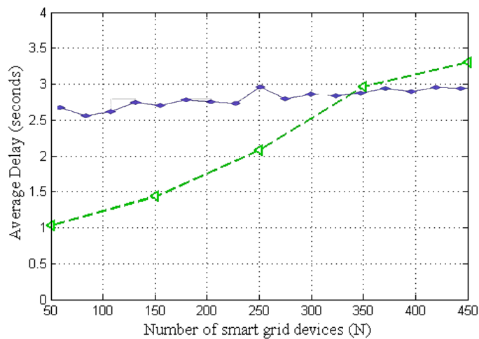
Figure 4.16: Average delay in seconds vs. Number of users for the smart meter application [54]
