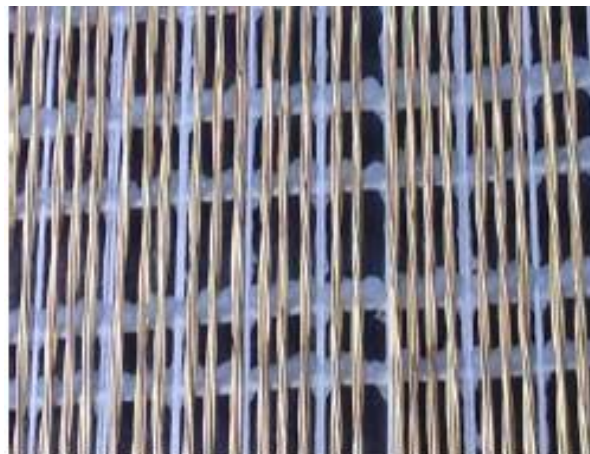
Figure 3: Medium-Density Galvanized Steel Mesh [41]
