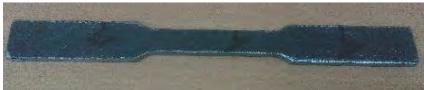
Figure 28: Steel coupon machined from Tube 4
