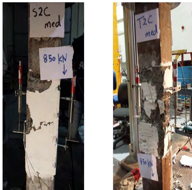
Figure 76: Observed damage of ISSSB and tied specimen (medium concrete)
