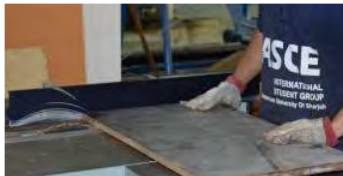
Figure 30: Making formwork in the manufacturing lab
