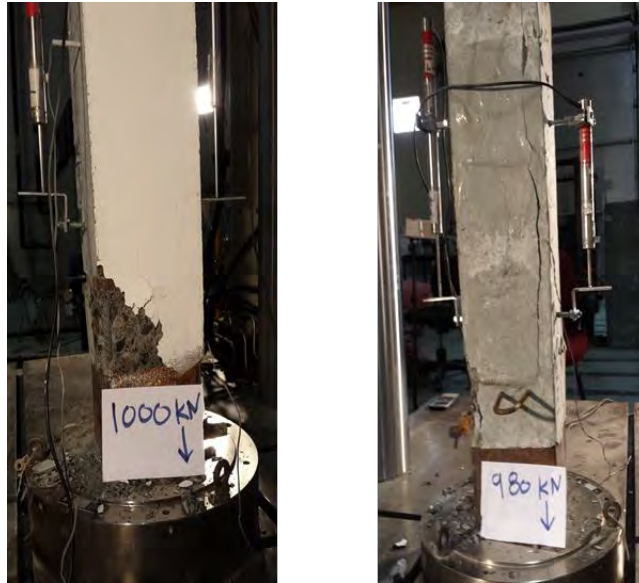
Figure 77: Observed damage of ISSSB and tied specimens (strong concrete)
