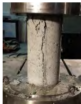
Figure 18: Testing of typical concrete cylinder
