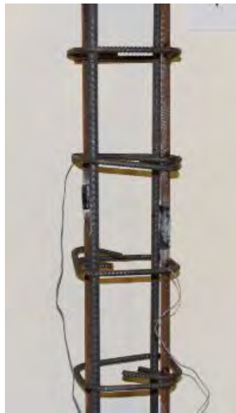
Figure 36: Connecting strain gauges to longitudinal bars to a tied specimen
