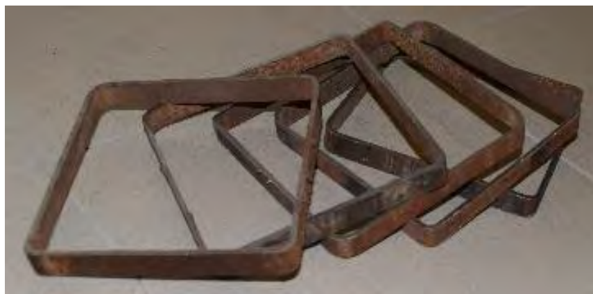
Figure 27: ISSSBs cut from steel tubes
