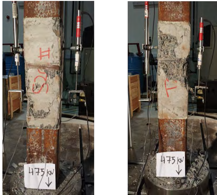
Figure 75: Observed damage of ISSSB and tied specimen (weak concrete)
