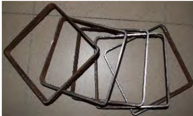
Figure 3: Internal Structural Steel Strip Bands cut from a square steel tube.
