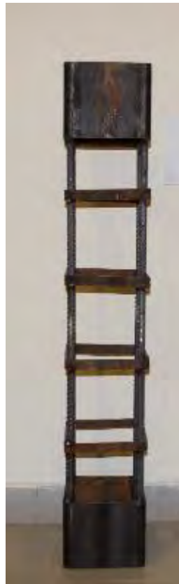
Figure 4: Steel cage for an RC column made with ISSSBs in lieu of ties.
