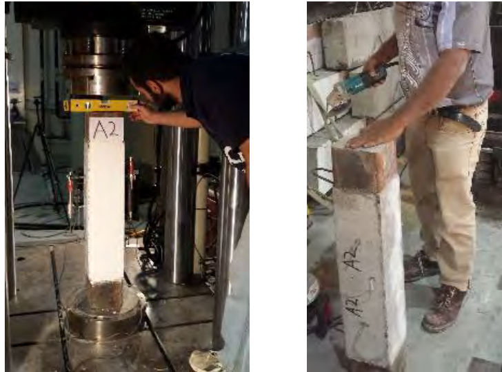
Figure 41: Smoothing specimen ends by electric grinding
