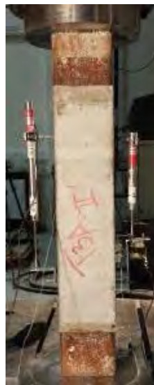
Figure 42: Connecting the LVDTs to the specimen
