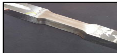
Figure 7: Geometry of the tensile test specimens at room temperature
