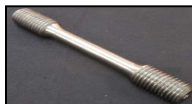
Figure 8: Geometry of the tensile test specimens at high temperatures
