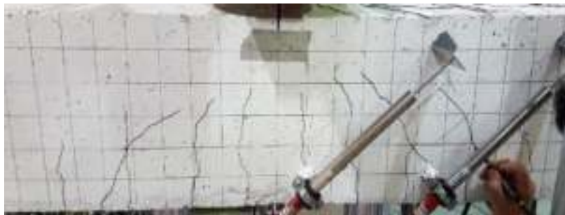
(c) Post-cracking stage
