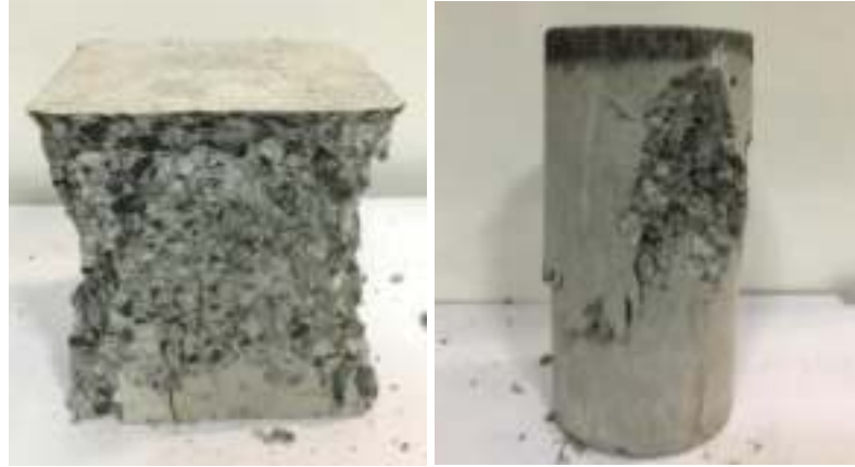
Figure 59: Typical cubes and cylinders failures of high f'_c specimens.
