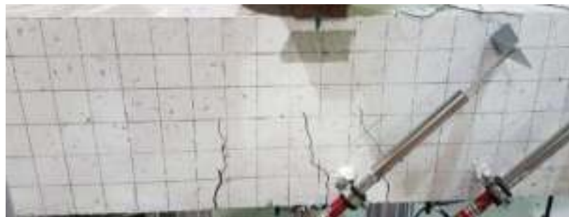
(c) Post-cracking stage
