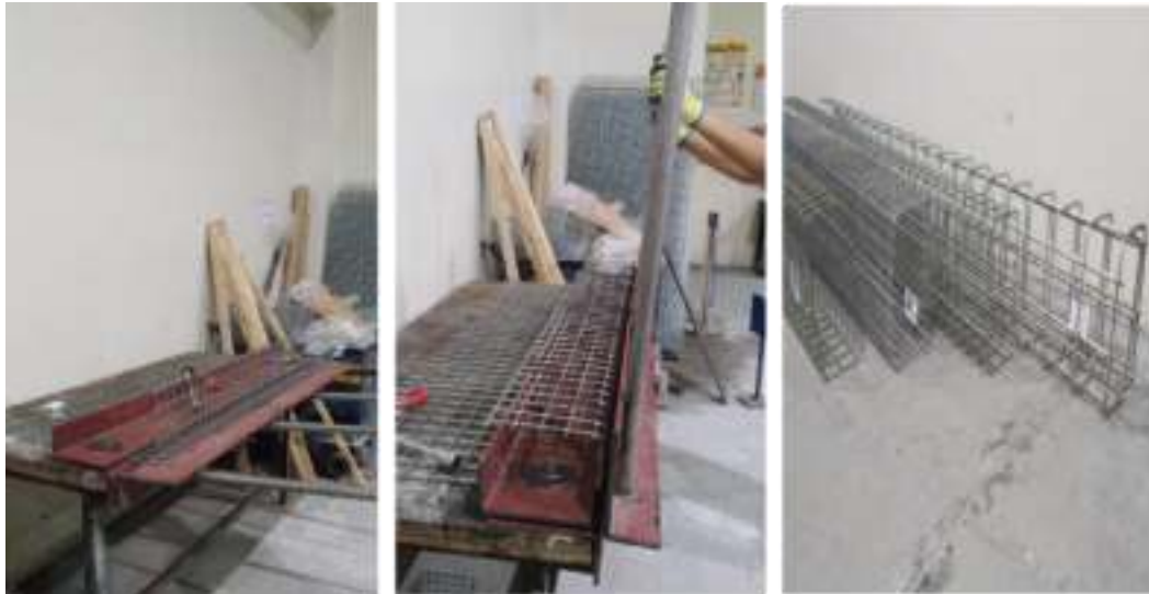
Figure 5: Fabrication of a steel cage from WWF sheet in the laboratory.
