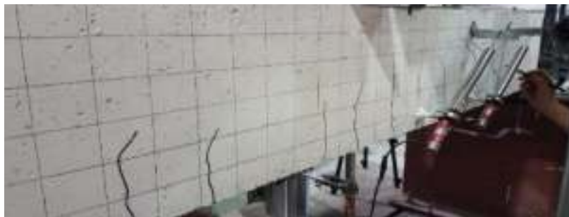
(c) Post-cracking stage
