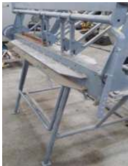
Figure 72: A metal brake machine used to bend thin metal sheets.
