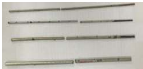
Figure 65: Tested wire specimens.
