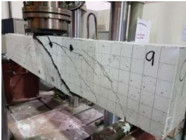
b) Typical shear failure.
