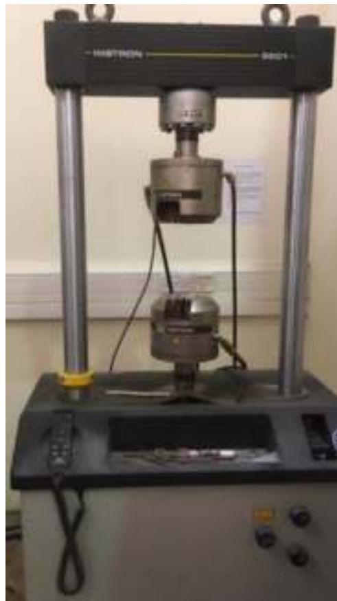
Figure 63: UTM machine used for testing the steel bars.
