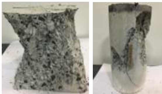
Figure 61: Typical cubes and cylinders failures of Group 3.
