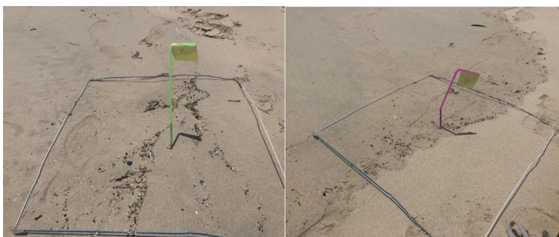
Figure 3.2: Sample collection along wrack lines
