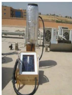
Figure 4. Thermosyphon effect used on PVT system [14].
