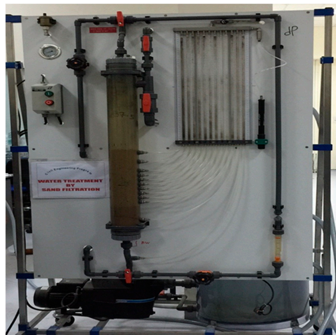
Figure 2. Sand filtration experimental setup.
