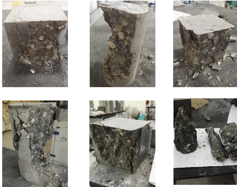
Figure B.6: Compressive strength failure for RA2 concrete mix
