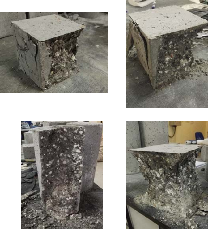
Figure B.5: Compressive strength failure for RA1 concrete mix
