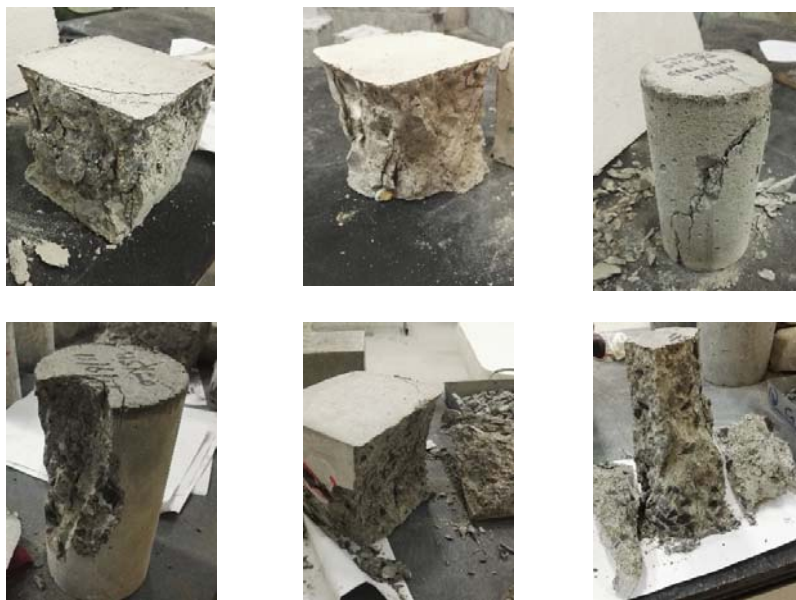
Figure B.7: Compressive strength failure for C45 ready-mix concrete
