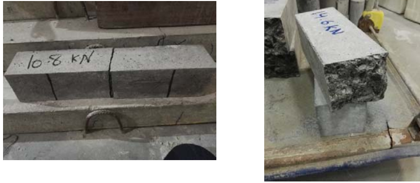
Figure 3.5: Flexural strength failure.
