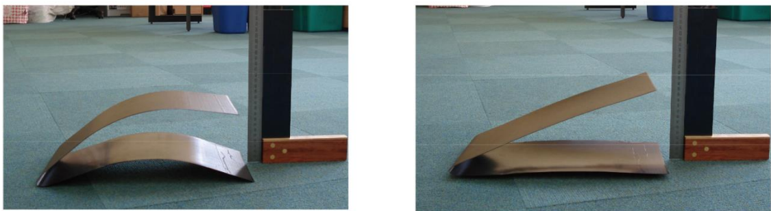
Figure 2-9: First stable configuration - Deployed Configuration (b) Second stable configuration - Extended Configuration for the variable camber trailing edge application [27].
