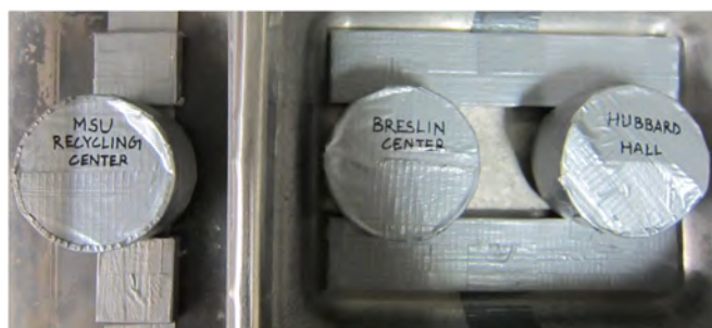
Fig. 5. Water sorption test setup.
